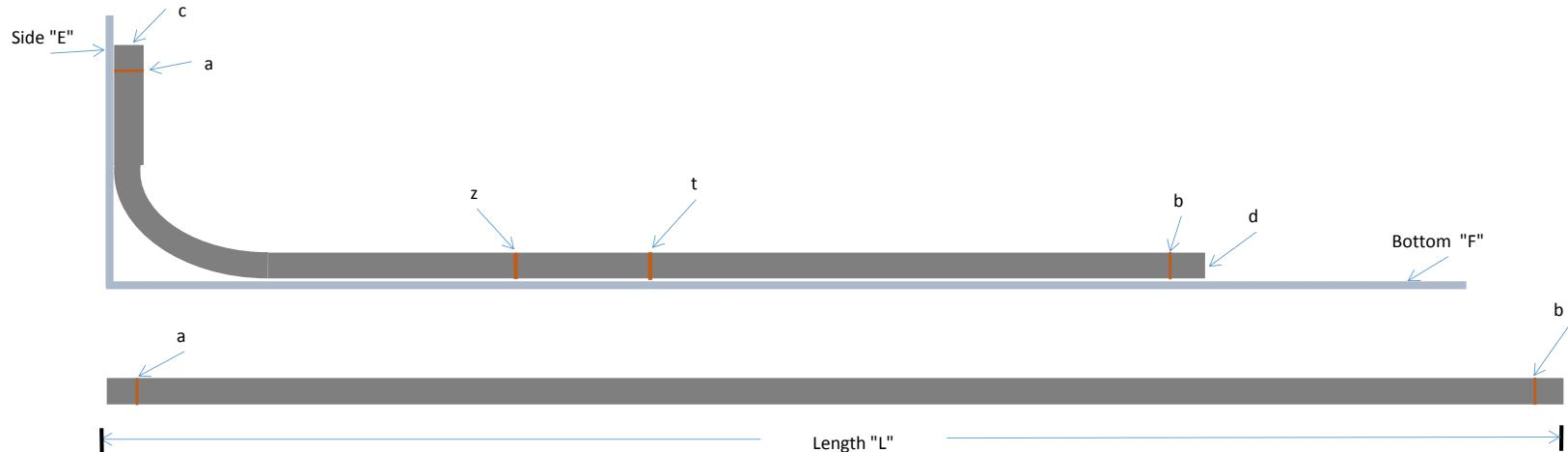
a = Place mark on conduit before installing conduit in bender
